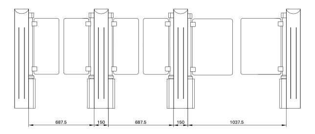
A wide variety of space-saving applications for pedestrians and wheelchair users can easily be implemented using a combination of modules with gates on one or two sides
