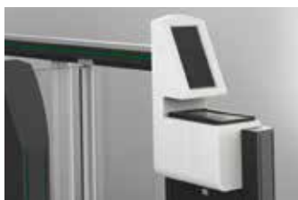
Entry kiosk and user guidance system detect personal data and guide users through the identification process.
